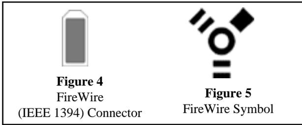
connector (see Figure 4) instead of the two main types defined under USB. However, just like USB, many companies have developed their own proprietary connectors for their FireWire-enabled devices.
