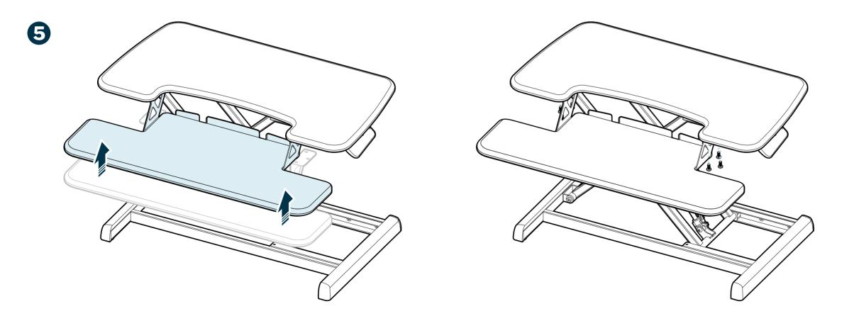
Line up the keyboard tray brackets with the pre-drilled holes on the underside of the top tier. Using a Phillips head screwdriver, screw in the pan head screws.
