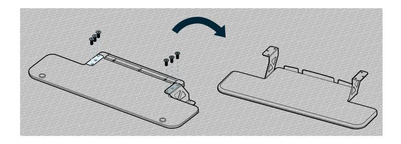
Flip over the keyboard tray so that the countersunk holes are facing up. Align the keyboard tray brackets as shown in the above illustration.
