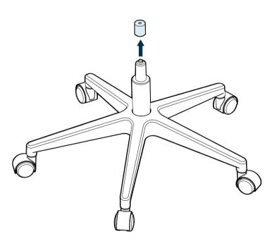
Place the piston into the center of the base with the smaller end pointed up.
