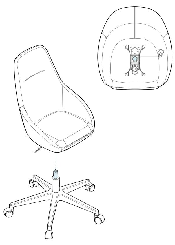
With assistance, take the chair seat and place the highlighted section of the mechanism onto the highlighted section of the piston.
